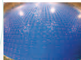
Looking into the Super-Kamiokande Detector nearly full of water.
