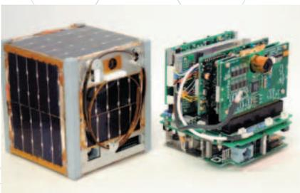
fig.1 External and internal view of CubeSat "XI"
