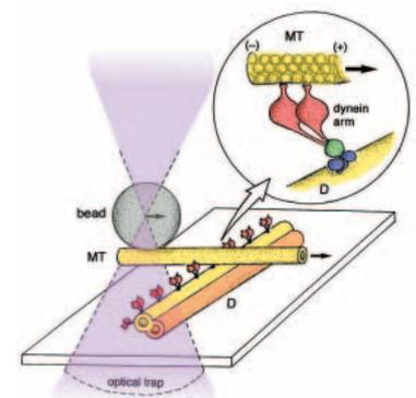
fig. Drawing showing the principle of optical-trap nanometry used to measure the force of a single dynein arm.
