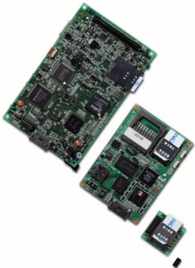
T-Engine is a standardized development platform for embedded systems. For distribution of middleware, a standardized platform is necessary. The photos are standard T-Engine, micro T-Engine, nano T-Engine, and pico T-Engine from the bigger size, respectively. Standard and micro T-Engines have been already released. Nano T-Engine is being built using all-in-one-chip microcomputer and pico T-Engine is being developed for smart RFID application.
