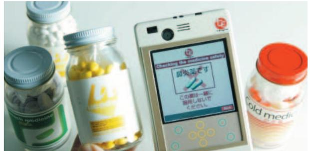
“Ubiquitous communicator” developed based on the T-Engine architecture by the Ubiquitous Networking Laboratory, where the author of this article, Ken Sakamura, Professor of The University of Tokyo, is the chair. Ubiquitous communicator is a terminal designed for individual communication and supports several communication methods. It works as a communicator with physical objects and a reader/writer of RFID and smart IC card.
