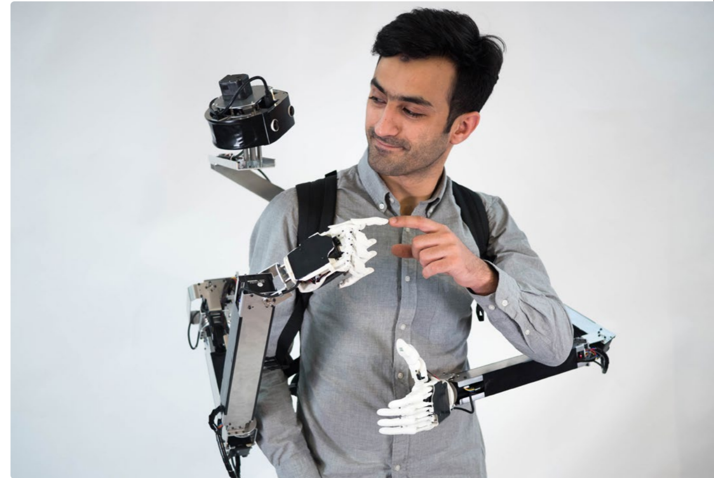
Remote operation enables two people in separate locations to share the same perspective and work in tandem. It is also a communication medium that increases empathy between the participants. (Photograph courtesy of the University of Tokyo, Inami/Monnai Laboratory & Keio Media Design)
