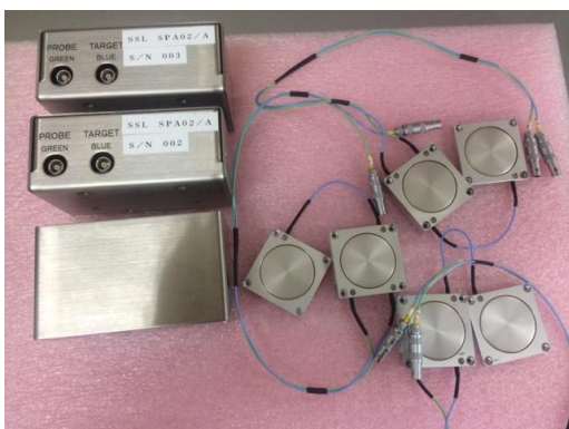
Fig.10 3Ch two plate cap. sensor & preamp
