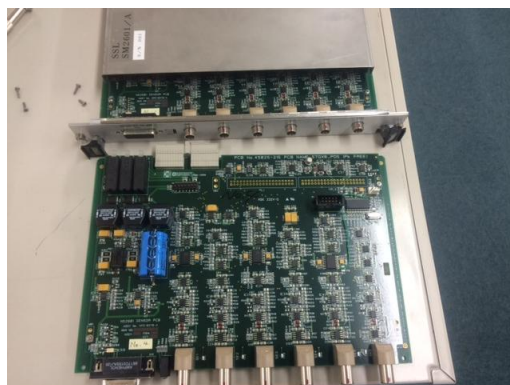
Fig 11 6ch two plate capacitance sensor amp
