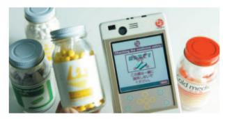
"Ubiquitous communicator" developed based on the T-Engine architecture by the Ubiquitous Networking Laboratory, where the author of this article, Ken Sakamura, Professor of The University of Tokyo, is the chair. Ubiquitous communicator is a terminal designed for individual communication and supports several communication methods. It works as a communicator with physical objects and a reader/writer of RFID and smart IC card.
