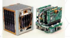
fig.1 External and internal view of CubeSat "XI"
