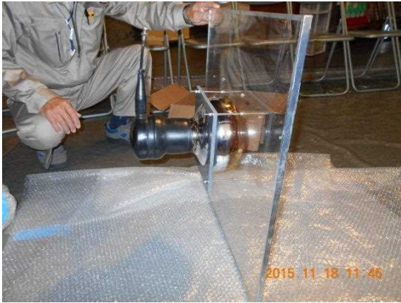
Figure 3. An 8-inch photomultiplier tube of the type installed in the Super-Kamiokande outer detector with its wavelength conversion plate.
